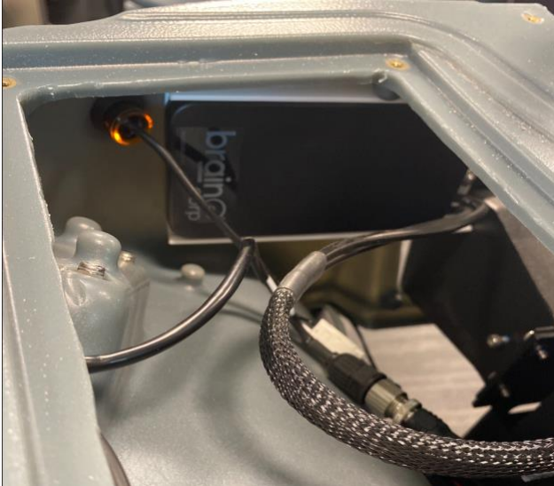
Figure 9: Antenna location underneath touchscreen display
